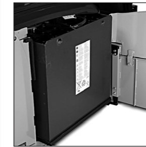
Lateral battery exchange
